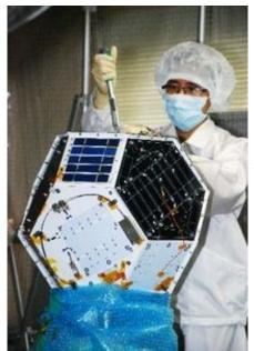
The Shin'en 2 satellite during assembly and testing. [Courtesy of Kyushu Institute of Technology/Kagoshima University]
